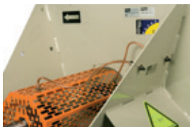
External lubricators to facilitate maintenance
