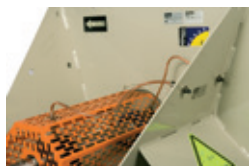
External greasers for ease of maintenance.
